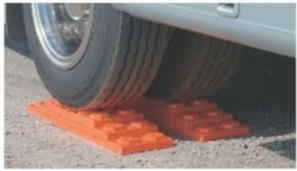
One block will raise your RV 1.5 inches, but when interlocking another leveling block to the stack or pyramid it will add 1 more inch. We recommend not stacking your levelers higher than 5 blocks (5.5 Inches).
