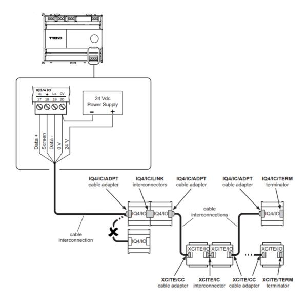
The IQ3/4 IO bus provides compatibility with I/O modules from the IQ4/IO and XCITE/IO ranges. Up to 192 I/O channels are supported on this bus.
