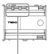
For use with Modbus, M-Bus, and/or XNC functionality. One port can also be used for an MSTP LAN of IQECOs.
