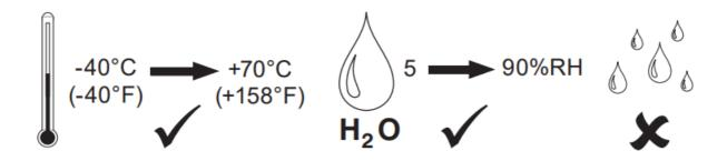
**Note:** For temperatures below 0°C (32°F) special care must be taken that there is no condensation on or within the unit.
