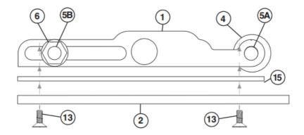
Safely invert the router and rest it on its top with the bridge and rods attached. Rest the baseplate on the flat of the router base ensuring that it's lined up with the bridge. Look between the bridge and baseplate and check the size of the gap. Slide the appropriate shims into the gap and line up the two x M5 tapped holes. Screw the baseplate onto the bridge.
