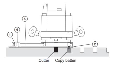
Clamp one guide batten on each side of the work piece, over lapping the ends. This will give a wider and longer platform to support the router. Depending on the depth of mortise and material being used, several cutting passes may be required in order to achieve the correct depth safely.
