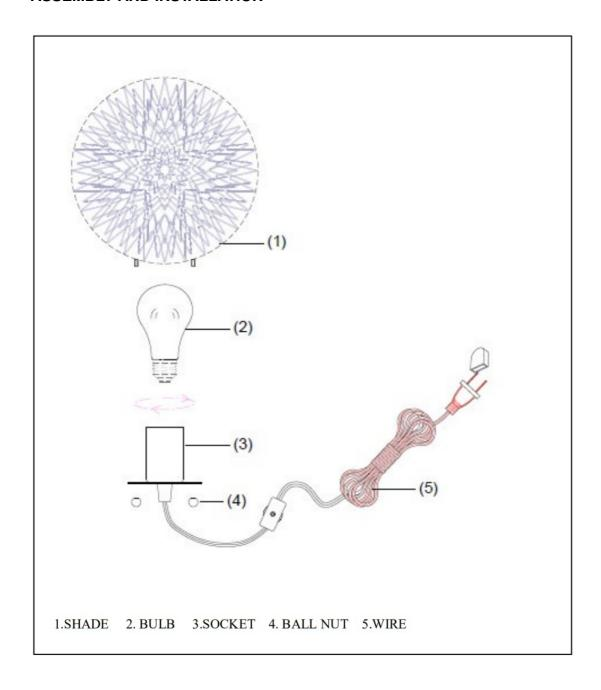
1. Loosen the ball nut(4) to take the socket out of the shade(1).
