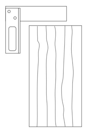
• Place the two boards to be joined with the face sides together.
