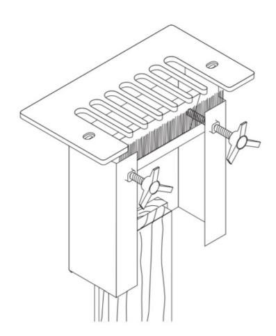
• Both boards should rest against the underside of the guide plate. Ensure both pieces of wood are firmly pressed against the left-hand edge of the jig: one piece against the offset stop, the other against the side of the jig
