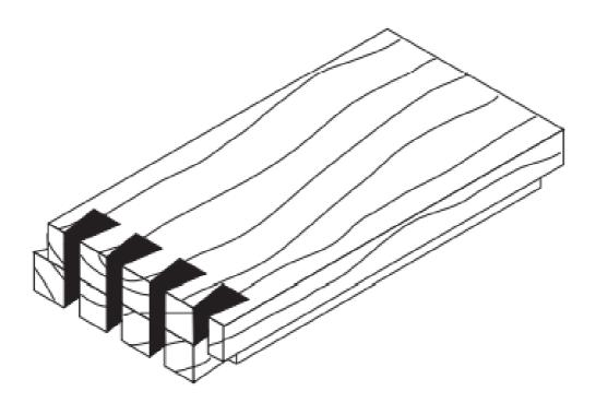
• Press the joints together. Glue as required.
