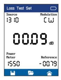
**Note:** This Example shows two OTDRs with PM and using the optical ports as CW sources for the light source. When using stand alone PM and LS, the PM will only have a single power meter port and the light source will have one or two ports depending on whether it is a dual or quad wave light source.
