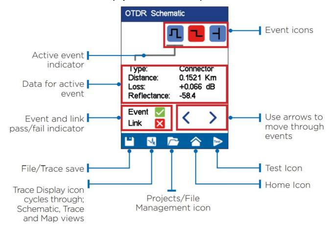
OTDR Trace Screen use Trace Display icon to cycle to the trace screen view.
