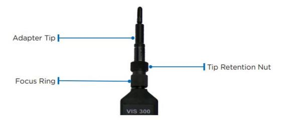
To remove a tip from the probe, grasp the probe tip and unscrew the tip retention nut. As oriented in the picture; rotate left to loosen and right to tighten the retention nut on the probe tip. Pull the tip straight up from the probe. To place a tip on the probe, ensure the lens is clean, slide the tip on to the end of the probe and tighten the tip retention nut. Do not over tighten the retention nut.
