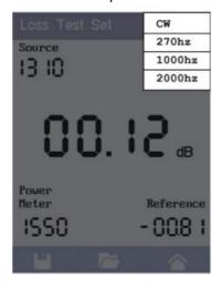
Touch the Power Meter indicator to show the power meter wavelengths available and select the appropriate wavelength for the test.
