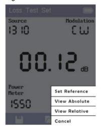
Touch reference indicator in the bottom right of the display and select, Set Reference to zero out the reference cord.
