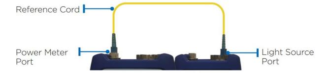
Plug one end of a reference cord into the light source and the other end into the power meter as shown below.
