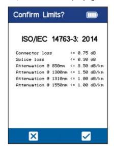
**Manual limits** may be selected on the OTDR Limits page. The following two pages of limits will be displayed to set limits/thresholds.
