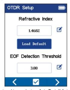
• Enough information has now been entered to conduct an Auto Test. If Auto is selected, the averaging time, range and pulse width will be automatically set based on analysis conducted by the OTDR. Select Manual and those parameters automatically set in Auto Mode will be available for adjustment.
