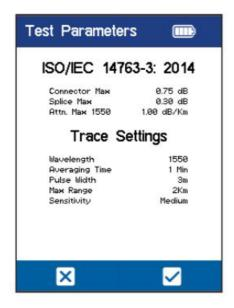
If the settings are correct, select the check box to start the test. A scanning status bar will be displayed, followed by a finding event message.
