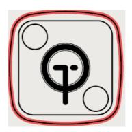
**Step 2**Press and hold the touch sensor for 3 seconds. The status LED will flash red.
