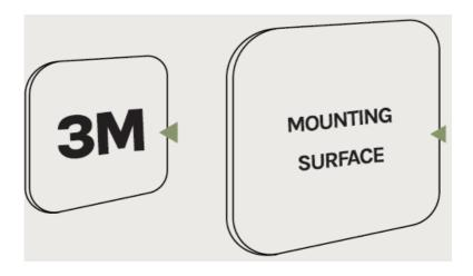
The 3M material is pre-mounted to the back of the Steel mounting plate. Take care to only remove the red plastic release tape and not the black foam adhesive.
