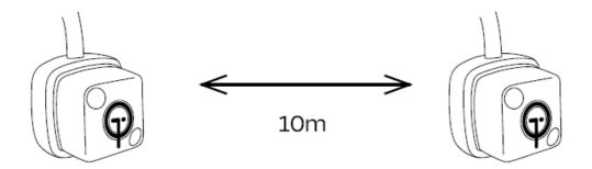
Recommended distance between Growcast to Growcast. When connecting and controlling the network with a smart device, we recommend that you are in the same room or within 10 meters of the Growcast to ensure the strongest connection.
