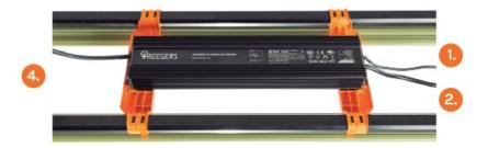
• Connect the cables (1 & 2) that exit from one end of the driver to the frame. The sockets for these are located underneath the powered side of the GL650W+ frame. When inserted, the ringlock of each cable socket should click and rotate when pushed in firmly. You can also connect the power cable (4.) to the single socket that exits the other end of the driver. Do not turn the power on yet.
