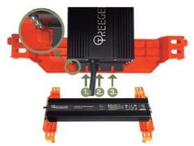
• Once the driver is secured to each of the driver brackets, attach the driver to frame assembly (as shown below), by clicking driver brackets onto the frame supports. Each bracket should be clipped into place, paying attention to the locating slots. Ensure the driver is positioned with the dimming (1.) and power cable (2.) facing to the correct side for attachment to the frame. Once in place, the driver will be secure with a little movement within the locating slots (3.)
