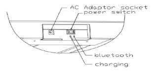
2. Press [ON/OFF] key on the indicator to turn on the indicator. The bluetooth LEDS on the indicator and the scale body both change from flashing to bright, indicating that the indicator and the scale body are connected successfully. The indicator will display a string of self-checking characters from 'PL===' to "PL—" "Pr—" "33333" for a few seconds and "——" then 0.00, now the scale enter the WEIGH mode.
