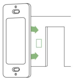
Thoroughly clean wallsurface. Remoue the paper fr om the adhesive strps on the back of the cradle
