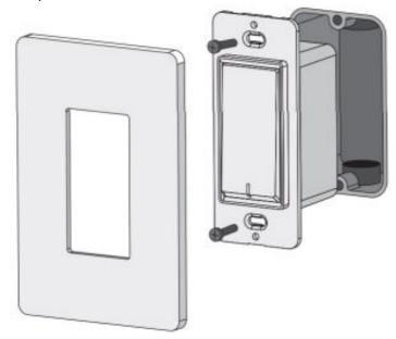
**Note:** Do not over tighten the screws, as it could restrict the operation of the switch.
