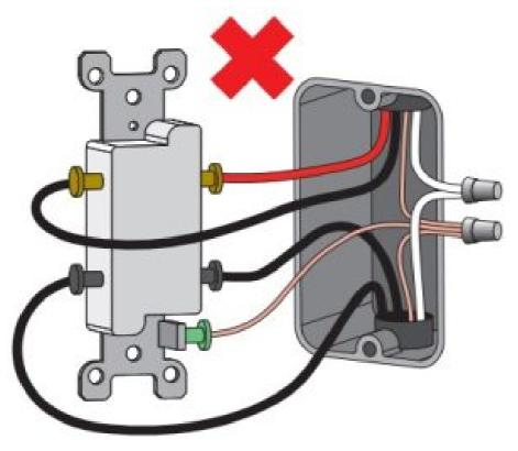
Screw the 4-way switch back to the wall, and unscrew one of the other two 3-way switches on the circuit that controls the same light.
