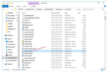
• Drag the aspnet\_regiis file into the Command Prompt then press the space bar and add the -i key. Then press the Enter key:
