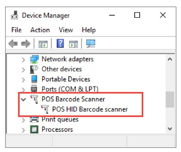
**Note:** If you don't see the barcode scanner as a HID device, scan the barcode below to appropriately program the scanner (see also the user manual at <a href="https://www.honeywellaidc.com/-/media/en/files-public/technical-publications/barcodescanners/xenon/xenon-ug.pdf">https://www.honeywellaidc.com/-/media/en/files-public/technical-publications/barcodescanners/xenon/xenon-ug.pdf</a>):
