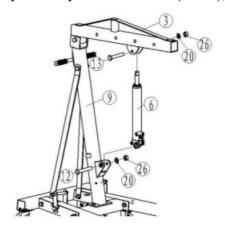
13. Push the boom extension (No.4) into the boom (No.3) and use a bolt (No.11), washer (No.20) and nut (No.26) to secure it at the desired load level. Using a bolt (No.16), washer (No.21) and nut (No.27), attach the hook and chain (No.8) to the end of the boom extension.
