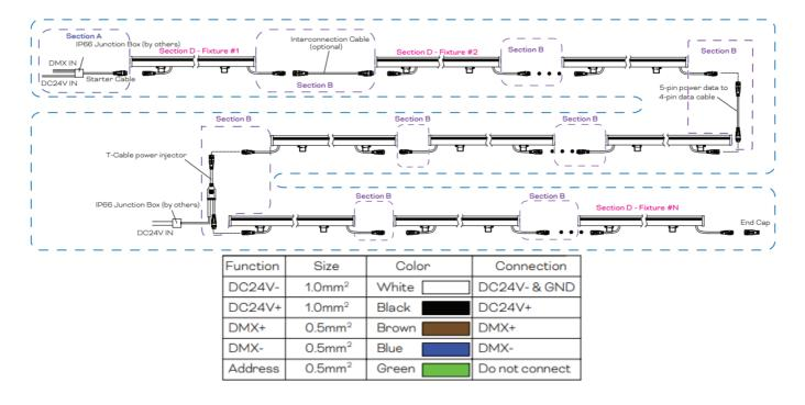
Data cabling from the DMX source to the Starter cable shall be Cat5e UTP or another cable type suitable for DMX communication.
