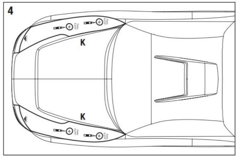
4K. Peel the backing from the included self-adhesive cutting templates. Install the templates on the vehicle body, aligning the edges with the existing body post holes and body lines.
