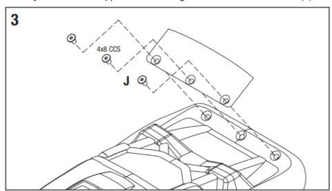
• 3J. Remove the 4x8mm CCS and plastic nuts (3) to remove the wing from the body.
