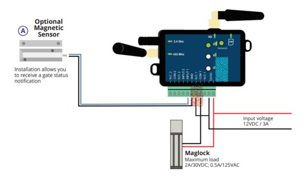
**Door or Gate Position switch** — Mount this on the door frame or on the gate in the desired location with the wire running to the input on the PAL controller, like shown above. When using two door or gate position sensors for double doors wire them in series with one leg of each switch running back to the controller for connection.
