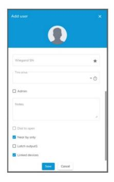
In this image, you will see that the "Nearby Only" box is checked. This enables a Bluetooth Credential, so that the user has to be in close proximity to the gate in order to open it. Leaving this box unchecked allows a user to open the gate from anywhere via a cellular signal.
