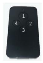
Buttons are designated 1-4, starting at the top and going clockwise around the remote. You can program all 4 buttons to the relay of a single PAL spider, or if you have multiple spider units, each button can be programmed to a differ-ent Spider Unit.
