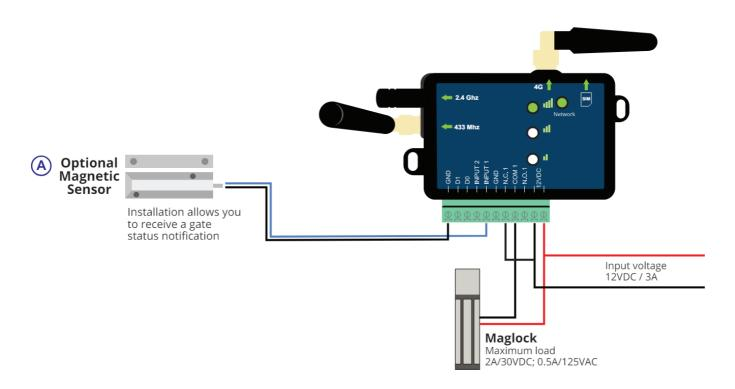
Typical wiring connection to a Gate:
