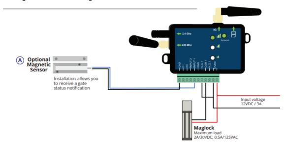
Typical wiring connection to a Gate:
