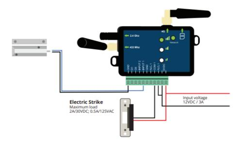
Door or Gate Position switch – Mount this on the door frame or on the gate in the desired location with the wire running to the input on the PAL controller, like shown above. When using two door or gate position sensors for double doors wire them in series with one leg of each switch running back to the controller for connection.
