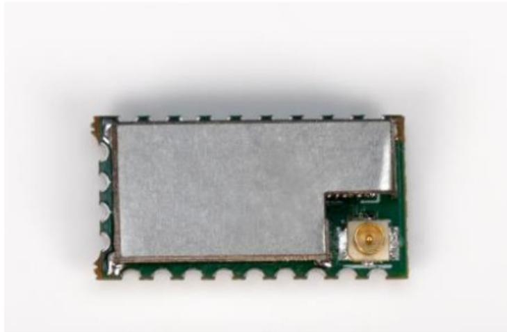
The JRD-1171 BLE module is a high-performance Bluetooth Low Energy (BLE) transceiver based on the Nordic Semiconductor nRF52840 SoC. It integrates a Power Amplifier (PA) and Low Noise Amplifier (LNA) to enhance transmission range and reception sensitivity. The module features a u.FL connector for external antenna support, making it ideal for applications requiring extended range and reliable communication.
