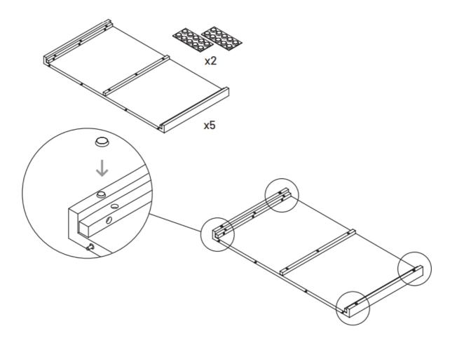
• Each Transformer Table comes with a package of 2 protective pads you will need to install onto each panel to prevent damage when they are being stored.
