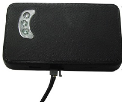
Figure 6 – Connect the Power Cable to the Transponder
