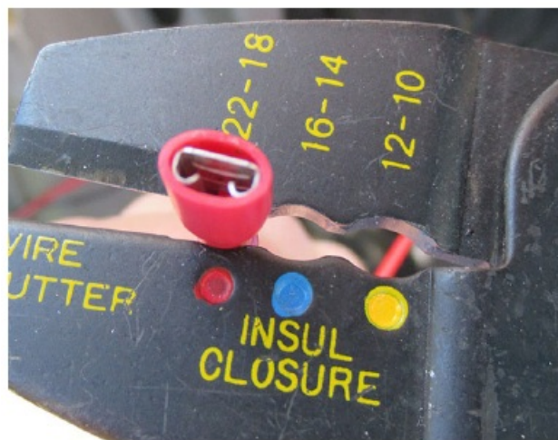
Figure 2 – Crimp Quick Disconnect onto Red Wire
