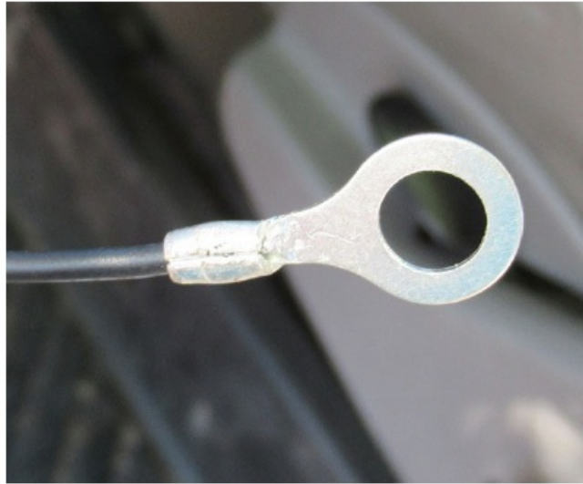
Figure 3 – Crimp Ring Terminal onto Black Wire
