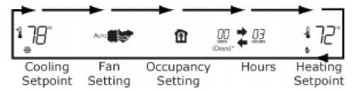
3. Press or to change the value of the currently active (flashing) selections. Repeat steps 2 and 3 for the desired settings.
