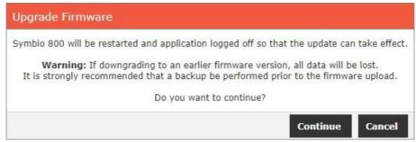
9. The controller will begin the firmware upgrade process. During this process the equipment will be stopped as the controller reboots. This process usually takes 5-10 minutes to complete. Symbio UI will automatically restart itself during the upgrade process. Do not unplug the USB cable.
