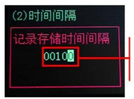
Press the second "SET" to enter the storage interval setting The upper limit can be set to 100 seconds/time
