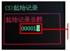
Press the third "SET" to enter the record Start point setting The upper limit can be set to 65101
