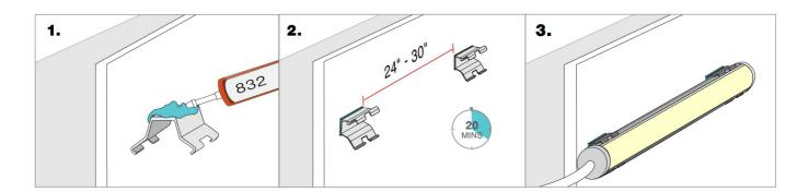
**NOTE:** 832 Silicone use in a well- ventilated area, 832 Silicone sold with Caulking gun. Do not use in any submersible applications.
