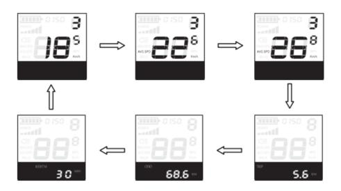
◆ Press and hold the "—" button to hold it down. After 2 seconds, the electric bike enters the power assist mode. The electric bike travels at a constant speed of 6 kilometers per hour. At the same time, the screen displays "WALK". Release the "—" button and the electric bike will immediately stop the power output and return to the state before the boost.
