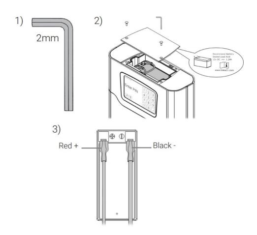
YUASA NP 1.2-12 12V, 1.2AH Valve Regulated Lead Acid Battery.
