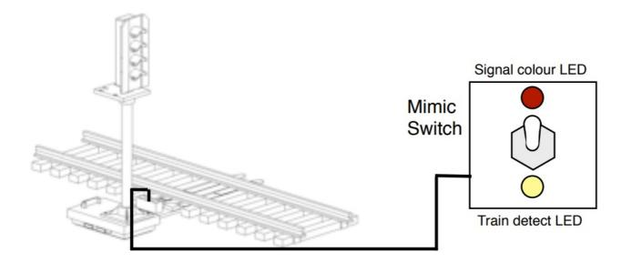
A Mimic switch connects to a Sensor Signal using just one wire and allows manual override of the signal as well as LEDs which show signal state and train detection, etc.
