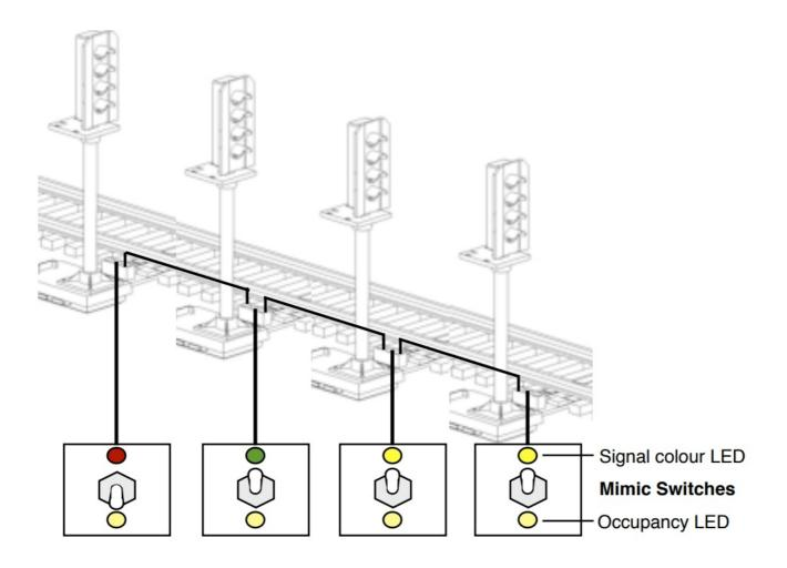
Mimic switches can be wired to one or more linked Sensor Signals using just a single wire. The top LED lights the same color as the signal. The bottom LED flashes as a train goes past a signal and lights continuously while a train is still in the following section to show block occupancy – ideal for a control panel to show where trains are on your layout.
