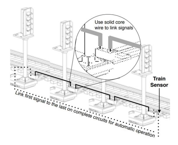
Wiring is easy because you just need one wire between each signal, the output of one to the input of the next one as shown. Always use Single core wire (1/0.6mm type is best) stripped 3-4mm at each end which just plugs into the signal sockets – you can either hide wires under your baseboard or run them on the top alongside the track – just like the real thing!
