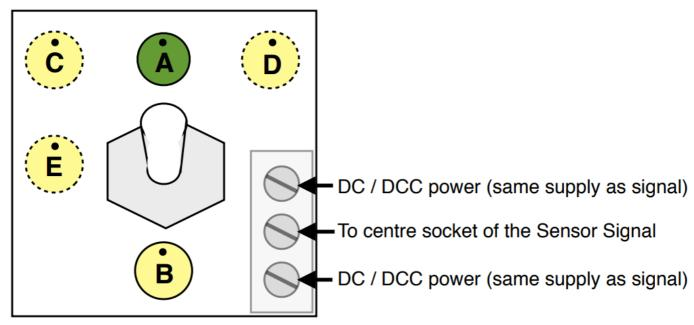
Using DCC to control a Sensor Signal
