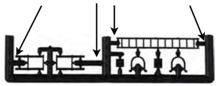
Mounting the signal on your baseboard You will need to drill a hole in your baseboard to clear the signal PCB we recommend a 6-8mm hole so that the signal can be lifted with wires still fitted if required. The signal can be free standing or held by suitable glue or double sided sticky pad.
