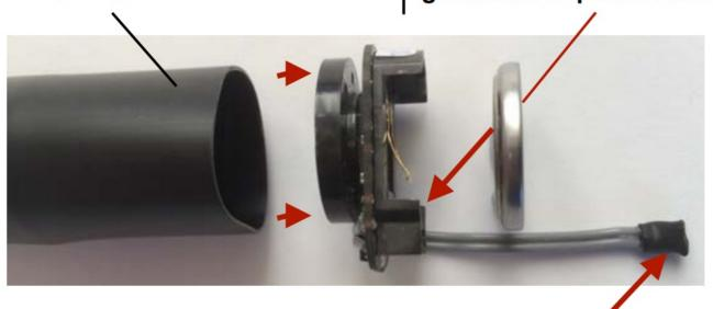
This is the Motion Sensor - always locate this *away* from speaker and not touching other surfaces in the model as it is very sensitive!
