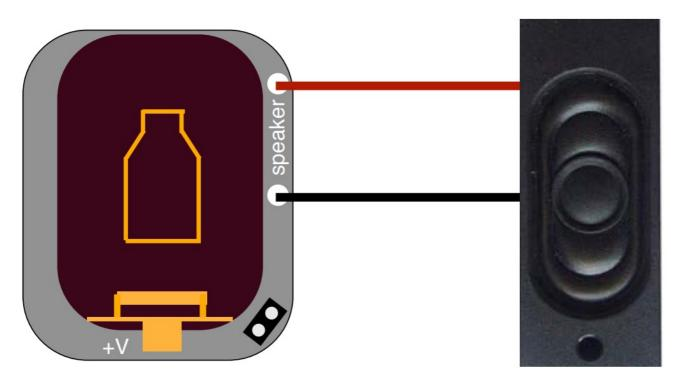
Note that you must disconnect the internal loudspeaker before connecting an external one otherwise you will overload the amplifier circuitry.
