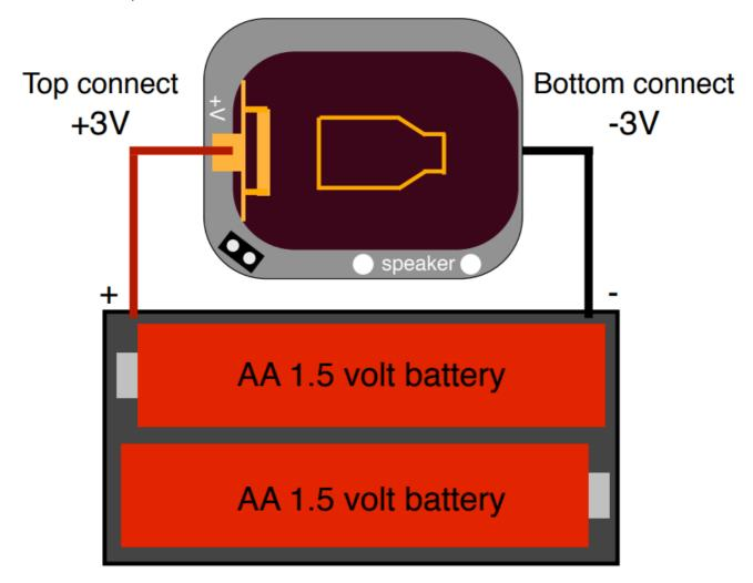
**WARNING**: Correct polarity & 3 volts MAXIMUM!
