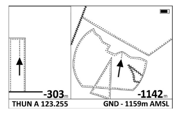
When you are inside an airspace, the two arrows indicate the shortest way out of the airspace. The displayed distance is then the vertical/horizontal distance to the edge of the airspace
