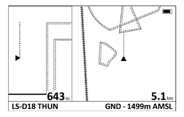
This is what the Airspace screen of the Maxx II looks like when you are approaching an airspace. On the left is the side view, and on the right is the top-down view. The numbers on the left show the vertical distance to the next airspace, and the numbers on the right show the horizontal distance to the next airspace.
