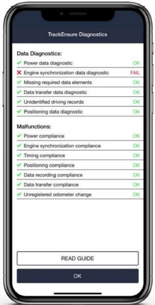
Malfunctions and Data Diagnostics indicate data inconsistency, failures or issues related to ELD. They can occur due to hardware or software failures, as well as external factors such as power failures, electromagnetic interference or physical damage to the device.
