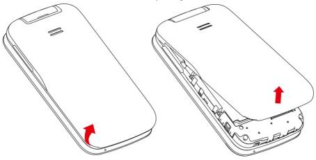
**Step 1.** With the device facing down, remove the back cover from the bottom left corner. Use your fingernail to carefully lift the cover away from the device body.
