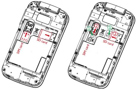
To remove the SIM card or microSD card, press down on the small plastic tab (①), then slide out the card (②). Do not use force or any sharp objects.
