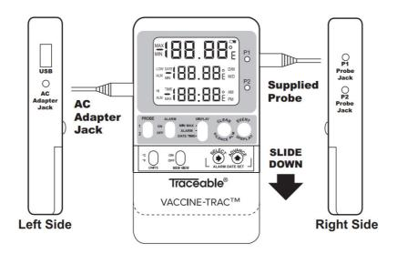
Probe labeled P1 must be plugged into the probe jack labeled "P1".
