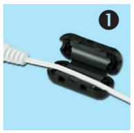
2. Loop the right end of the cable under the suppressor and back up again laying the cable along the center of the suppressor.
