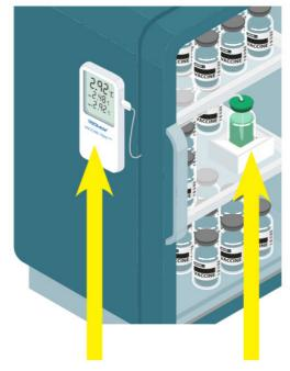
Place data logger on OUTSIDE of refrigerator/freezer Place probe bottle and holder INSIDE of refrigerator/freezer on middle shelf
