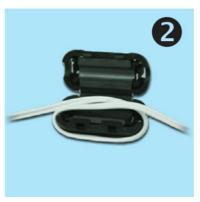
3. Carefully, snap two halves together with looped cable routed through the center
