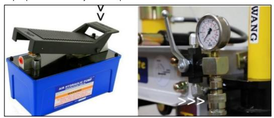
2. With pump in its upright, horizontal position, remove the oil filler plug located on the top plate of the reservoir.
