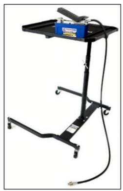
4. Depress the pump pedal end marked "pump "position for 5 seconds to allow the pump to operate, stop depressing the pedal at 5 seconds then leave the pump and hose for 10 seconds for trapped air to settle. Repeat this procedure 5 times, then check oil level as described in step 2.
