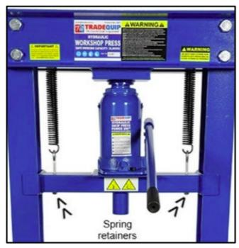
2. Remove the bottle jack base mount screws and gently remove the jack from the frame and place on a suitable work bench for the bleeding procedure to continue.
