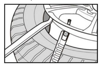
2. Adjust the sensor angle according to the angle of the hub and install it
