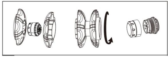
2. Fix in the new battery (positive+ side facing up).
