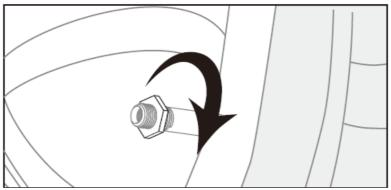
2. Install the sensor onto tyre valve clockwise.
