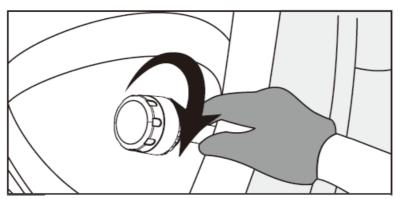
3. Use the spanner provided to screw the hex nut to the sensor and tighten it.
