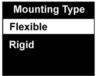
As a basic "rule of thumb", unless a machine is bolted down to a concrete floor, its mounting should be considered as being flexible.
