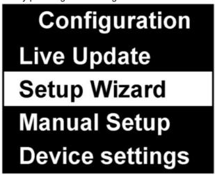
Moving up and down the menu is achieved by pressing the left (up) and right (down) buttons which causes the menu item to be highlighted. Pressing the circle button will select the highlighted menu item. Left and right arrow buttons can be used to move backward and forward through the menus.
