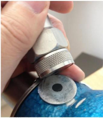
N.B. for best results the sensor should be placed gently onto the measurement point by "rolling" the magnet onto the machine.
