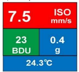
Taking a reading causes the overall vibration numbers and temperatrue screen to be displayed as shown in the example screen left. Note: Temperature will not display if a standard low power accelerometer without temperature (p/n A9100) is used.
