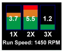
N.B. in order to perform a vibration analysis it is important that the running speed of the machine is entered correctly. This can be done with the "Setup Wizard" as described in Section 2.3.1 of this user guide, or by using the strobe attachment (see Section 5.1) The frequency ranges of the VA bands are based on the following multiples of running speed 2:
