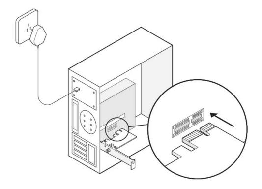
d. Locate an available F\_USB connector and carefully plug the USB cable into it.
