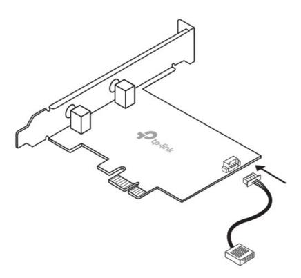
c. Locate an available PCIE X1 slot and carefully insert the adapter.
