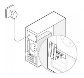
D. Replace the case panel, plug in the power cable and turn on your computer.
