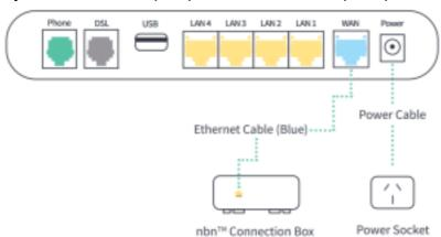
**Important:** These nbnTM technologies require two devices to work. Refer to the HFC or FTTC guides provided by nbn for instructions on how to set up the nbnTM Connection Box.
