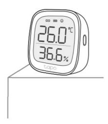
(The installation height should not be higher than 2 meters.)
