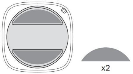
b. Magnetically attach the sensor to metallic surfaces.
