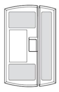
Choose where you'd like to install (but don't affix it yet). Place the magnet near the edge of the door or window that moves. **Note**: The recommended height is below 6.56 ft (2 m).
