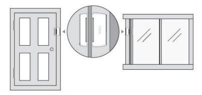
Align the magnet and sensor with no more than 0.39 inches (10 mm) between them. Peel the backing from the attached tape and press the sensor and magnet into place.
