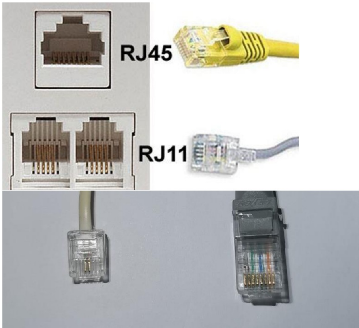
Figure 8: RJ45&RJ11 Pairs Figure 9: RJ11 in real RJ45 in real Table 1: Comparison between RJ45&RJ11
