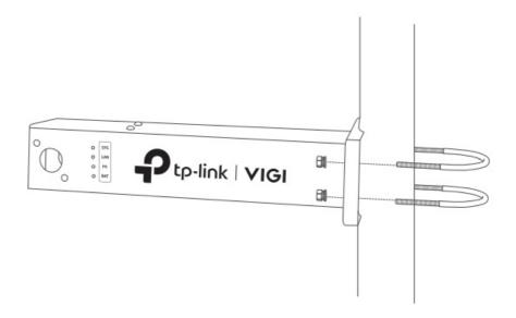
**Tip:** Determine the direction according to a compass or mobile phone compass software, and adjust the orientation of the bracket to obtain the maximum solar energy.
