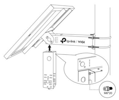
2. Install cameras on the vertical mount using camera mounting screws (M4\*20). For PTZ cameras, use PTZ camera connector mounting screws (M6\*20). Different types of mounts have varying access methods, and the corresponding type of bracket should be selected for installation according to the actual situation of the device. The installation hole diagram of the load at the end of the vertical mount is as follows:
