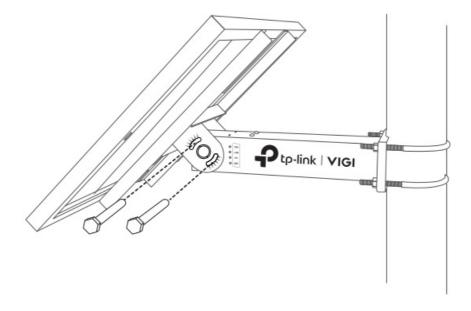
Step 5. Install the vertical mount and cameras
