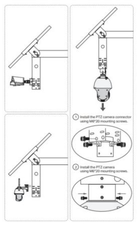
**Note:** If the product is used in a windy area, it is recommended to tie VIGI 5-Series cameras directly to the pole to reduce the impact of strong wind on the image quality of the camera.
