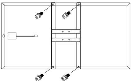
2. Install the angle adjustment bracket to the solar panel bracket using four M8\*20 mounting screws.
