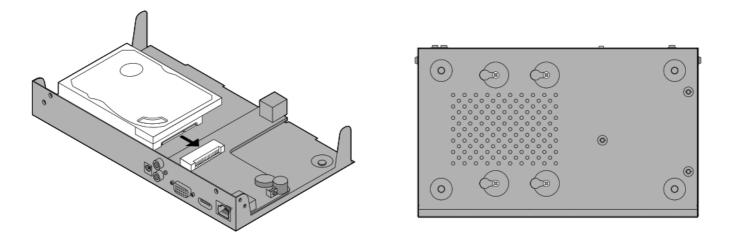
4. Flip the NVR upside down and fasten the HDD screws. Replace the cover and fasten the screws of the NVR.
